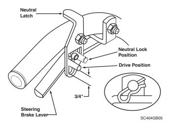
Figure 6-1. Steering Control Rod Adjustment
